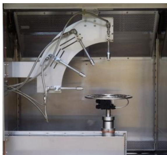
Figure 2. High pressure steam nozzles and the specimen rotator
